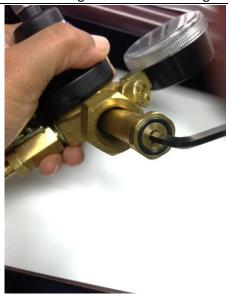
Retighten the retainer completely to prevent CO<sub>2</sub> leaks.
