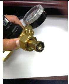
Seat the new or cleaned ring fully into the recessed space. Invert reused rings before installing. The fit will be snug.
