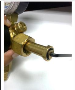
Use a 5/32" hex key to remove the retainer and gain access to the ring.
