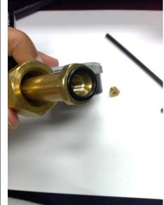
Gently pry the ring up and out of the recessed space in the nipple.
