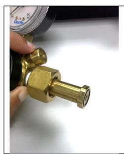
Taprite inlet nipple O-rings and flat rings can be easily replaced.
