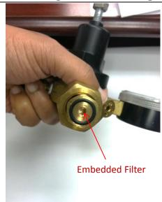
Note that the internal filter should remain in place during replacement.
