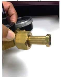
The tightened retainer will sit just below the top of both the O-ring or flat ring and the outer brass lip.
